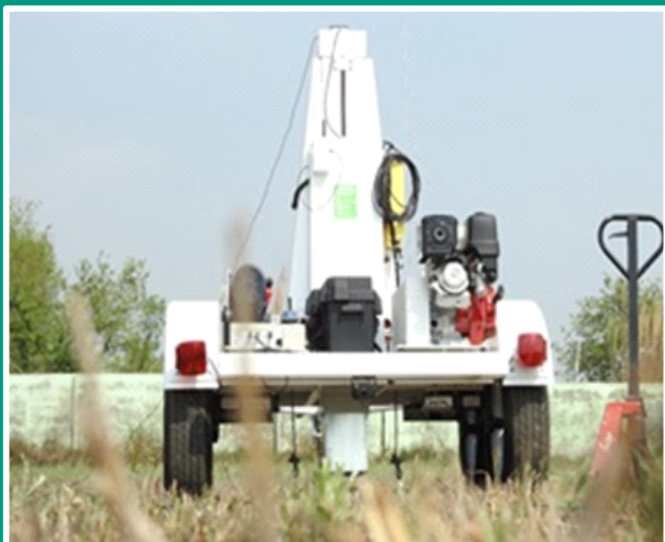
ESS1000 WITH 950-1000 Pound hammer (seismic energy source)
